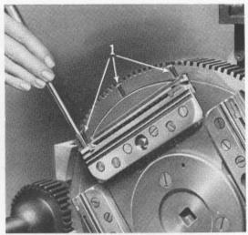
FIG. 34-1. View of method of changing mold liners.
