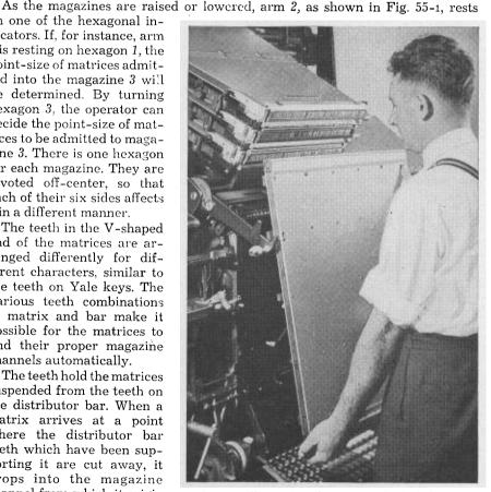
FIG. 61-1. Illustration showing method of changing magazines.
