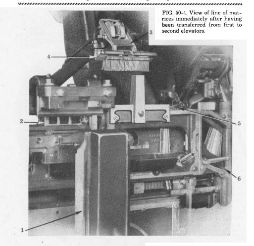
keeps the first elevator from descending full distance, all of the lines being cast in the auxiliary position. This device is called the Simple Two-Letter Attachment.
