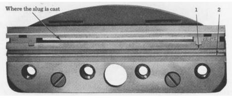
FIG. 30-1. Note the upper and lower rails (indicated by arrows 1 and 2 at the right) against which the matrices align to cast in the regular or auxiliary position as predetermined in the assembling elevator.
