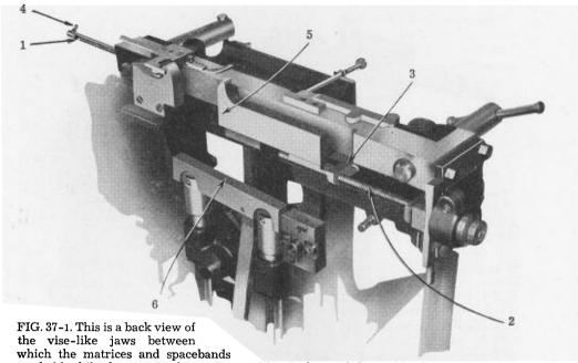
are held while they are in the casting position in front of the mold. The mold disk, of course, is not shown here as it would make this view impossible.
