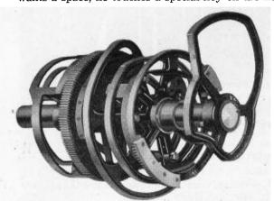
FIG. 3-1. The cams assembled on the shaft actuate and control most of the mechanical actions of the Linotype. A one-third horse-power motor drives the entire machine.
