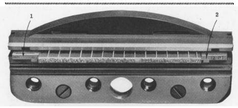
FIG. 29-1. The length of the mold slot (and the length of the slug) is determined by the length of the piece of metal, or liner, 1. If the point size of slug is to be changed liners 1 and 2 are removed and liners of different thickness inserted (Fig. 34-1).
