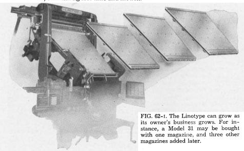
Magazine additions, as indicated in Fig. 62-1, can be made in the composing room by any operator. No dismantling or discarding of old parts is necessary, nor is the assistance of an expert machinist required.
