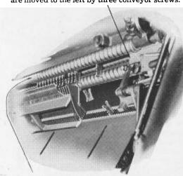
Each matrix is moved along by these screws to a point at which the corresponding teeth on the bar are cut away and cease to support it. It drops at this point into the correct channel of the magazine below.
