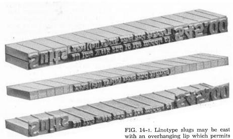
large characters to lap over one or more adjacent slugs. The upper section of this illustration shows such a combination, and the lower, the two slugs separated. The mold in which they are cast is shown in Fig. 33-1.
