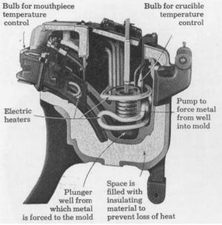
FIG. 41-1. Cross section of Linotype electric pot.
