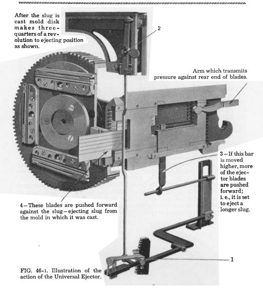
vary the length of the line of type on the slug in accordance with requirements.
