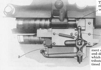
This cam causes periodic right-and-left motion of small vertical arm 1.
