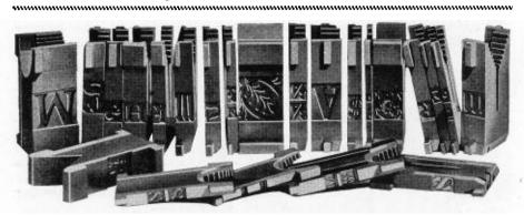
FIG. 5-1. A few matrices of a wide variety of characters commonly used in printing. They are made in sizes from 4 point to condensed 60 point.
