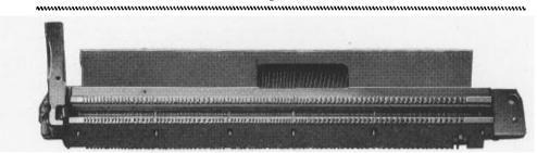
FIG. 23-1. An assembled escapement.
