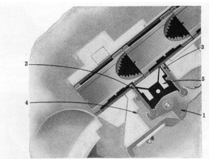
FIG. 21-1. The escapement mechanism.
