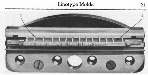
FIG. 31-1. Recessed mold.
