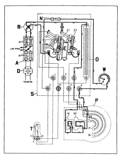
Diagram No. 6 explains the mouth and throat heater circuit only. Note that this circuit does not pass through the magnet switch E, and, therefore, the heating of the mouth and throat of the pot is not controlled by the action of the temperature control T or the position of magnet
