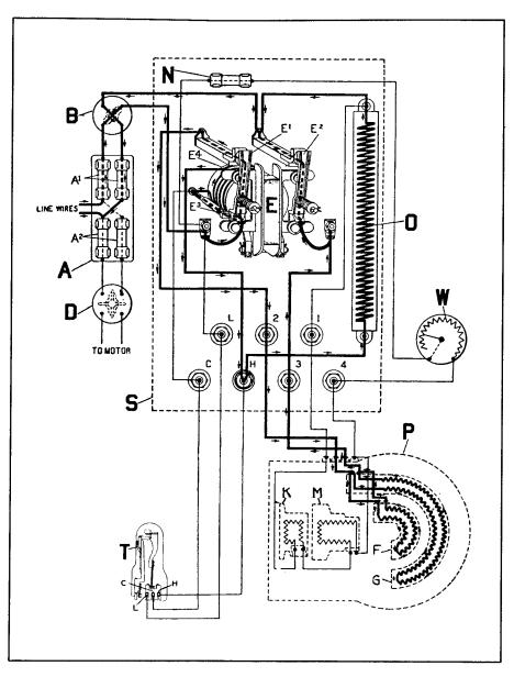
When magnet switch E closes, the contact that is made at E-3 short circuits the temperature control circuit and relieves it of carrying current. A circuit is still maintained through coil E-4 by contact E-3, which holds the magnet switch E closed.
