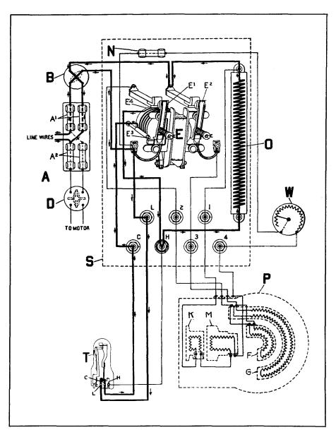
This diagram shows switch B turned to the on position. Current immediately flows from the line through switch B to terminal L on the panel and then to temperature control contacts L and C and back to terminal C on the panel, then through magnet switch coil E-4 to terminal H on the panel. Current then passes through
