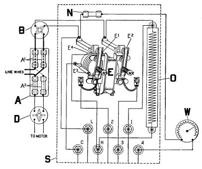
Control Panel Wiring, Fig. 6
