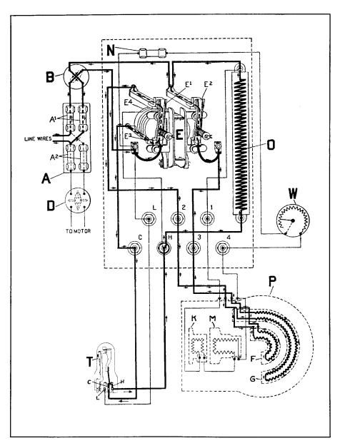
This diagram shows the current when the temperature of the metal has just reached 550° F. Note that the temperature control roller contact is touching contacts C and H, which short circuits magnet switch coil E-4. No current will pass through the magnet switch coil, because
