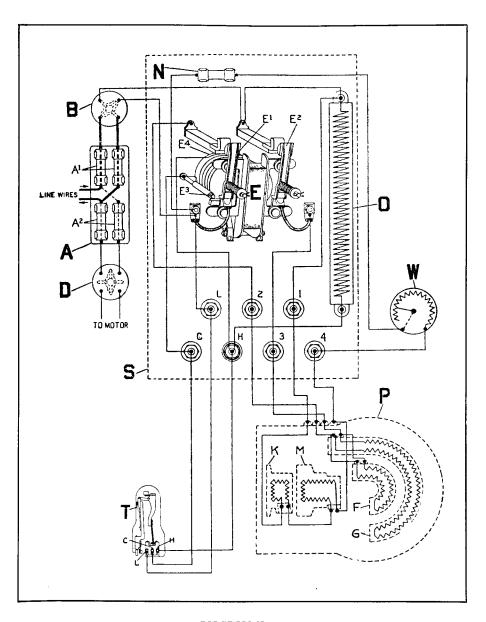
When magnet switch  $\boldsymbol{E}$  opens, it disconnects the crucible heaters  $\boldsymbol{F}$  and  $\boldsymbol{G}$  from the circuit and the metal begins to cool. This diagram is like Diagram No. 1 except that switch B is shown in the on position and the temperature control roller contact is touching contacts C and H instead of contacts C and L.
