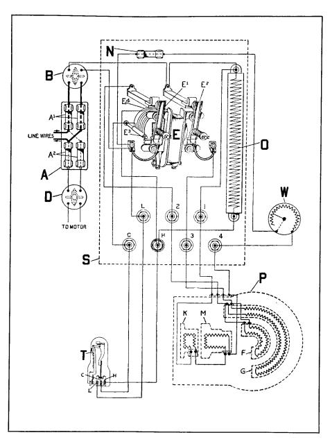
This diagram shows the electric connections of the pot with the pot control switch B turned to off position and the Linotype metal cold. Current cannot pass switch B, therefore the whole pot is dead. Note that the temperature control
