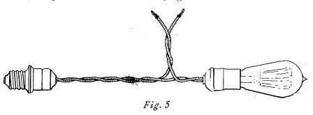
Connect the lamp cord to the attachment plug and the keyless socket in the ordinary way, then cut one of the two strands of the lamp cord a few inches from the lamp socket. Remove the insulation for one inch from the two ends of this strand of the lamp cord and twist the wires tightly. (See Fig. 5.)
