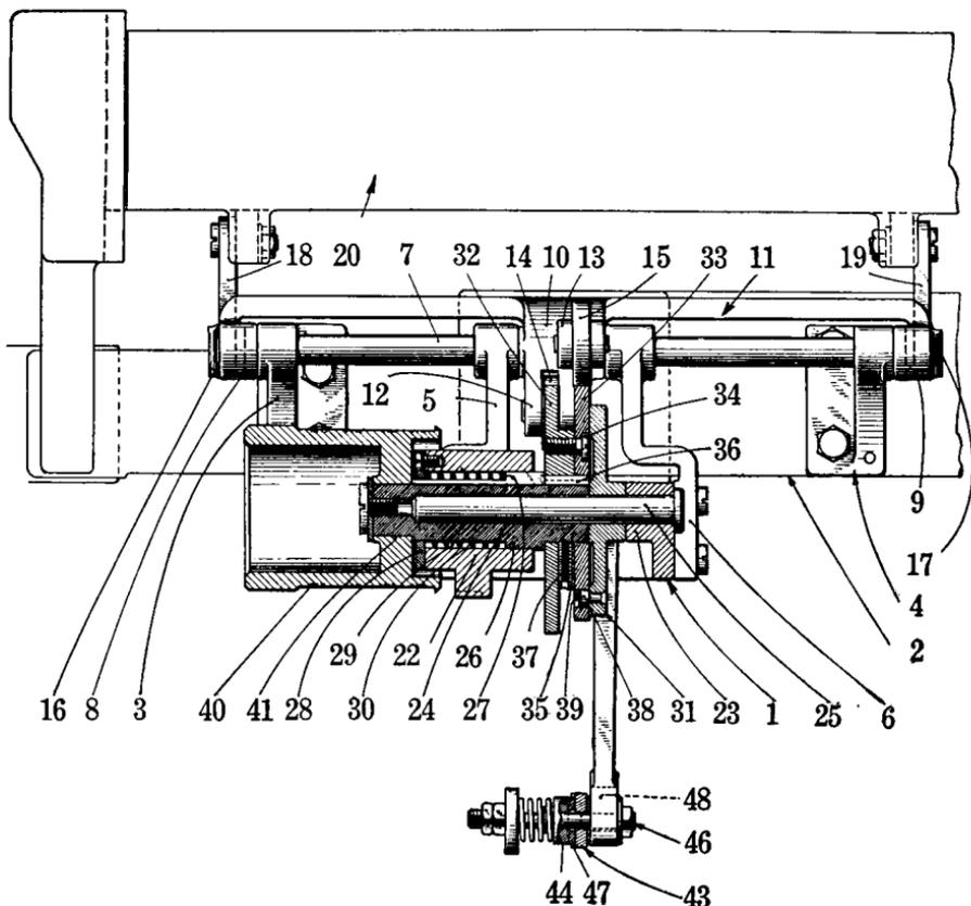
FIG. 3-26. Plan view of Model 31-32, 72-90 character Channel Chooser, shown partially in horizontal cross-section.
