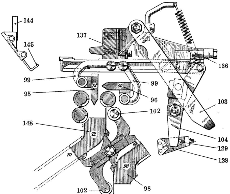
FIG. 14-26. View similar to Fig. 13-26, showing diagram of channel entrance unit and distributor bars in position for 72-character operation.
