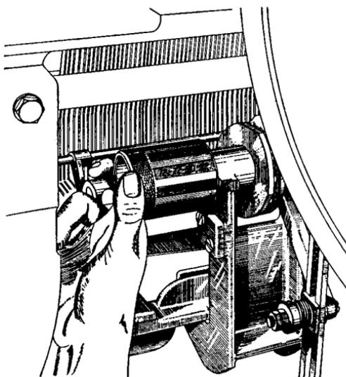
FIG. 1-26. View showing the Channel Chooser and method of setting.
