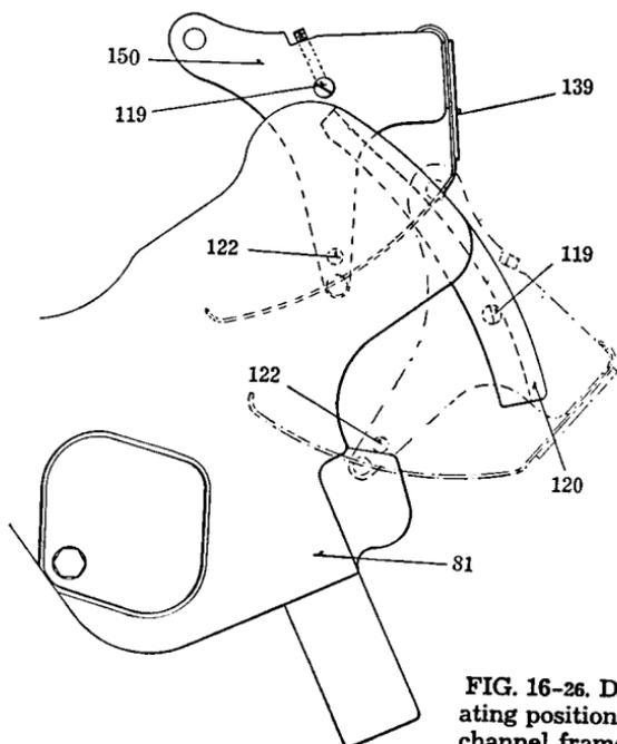
FIG. 16-26. Diagram of channel frame in operating position. Dotted lines indicate position of channel frame when opened for inspection.
