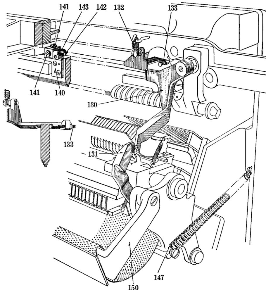
FIG. 17-26. Perspective view from the rear of the machine, showing the distributor bar retaining lever cam 131 contacting the distributor bar retaining lever 130; and also additional mechanism for securing distributor bar in correct operating position.
