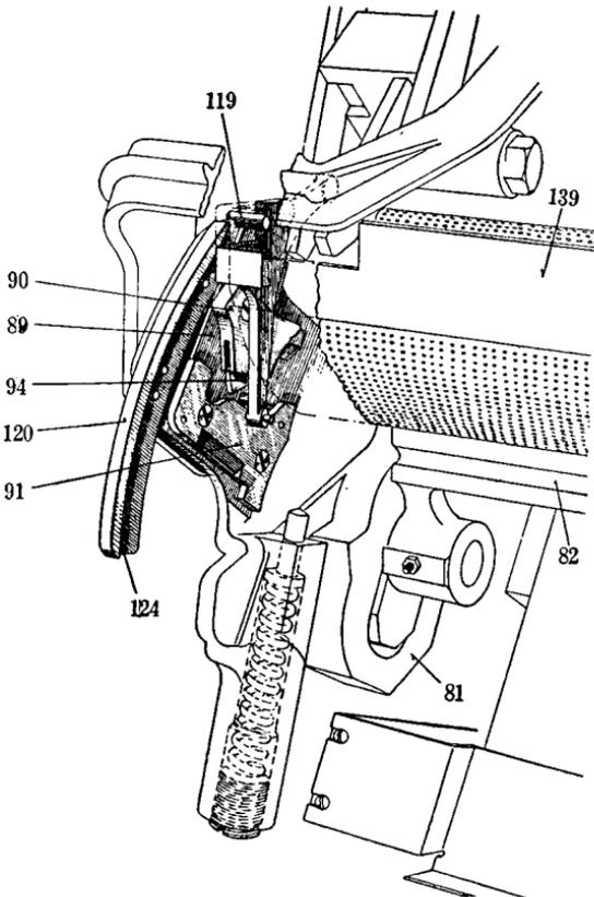
FIG. 12-26. View of channel frame and cam plates in operating position.
