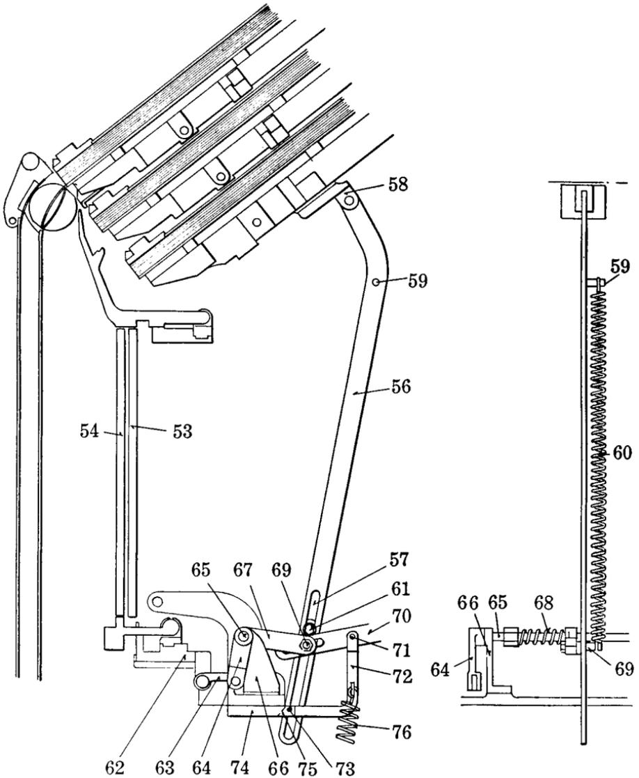
FIG. 6-26. View showing setting of the Keyboard Rod Lever Slide Shifting Mechanism on "Two-in-One" Models 8 and 14, when set for *Standard* arrangement of magazines.
