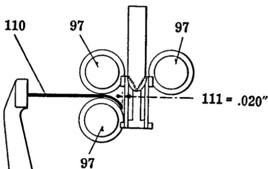
FIG. 15-26. Diagram of matrix guard safety mechanism, indicating clearances which are necessary for efficient operation.
