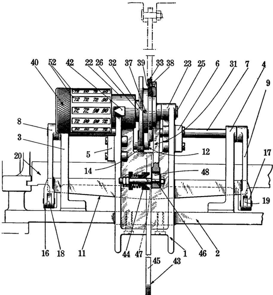
FIG. 4-26. This diagram represents a rear elevation of the automatic Channel Chooser mechanism on Models 31-32 machines.
