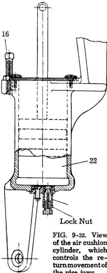
FIG. 9-32. View of the air cushion cylinder, which controls the return movement of the vise jaws.
