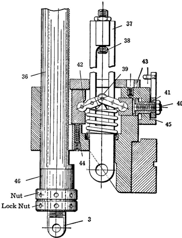
*To adjust Shoe 50, Fig. 12-32*—Adjust screw 61, Fig. 13-32, until the center of shaft for roller 64 is  $8\frac{1}{8}$  inches from the center of the main cam-shaft. This is shown in Fig. 4-32. Then adjust shoe 50, Fig. 12-32, so that there is approximately  $\frac{1}{8}$  to  $\frac{3}{8}$  inch between lever 52 and shoe 50, as shown at 56.
