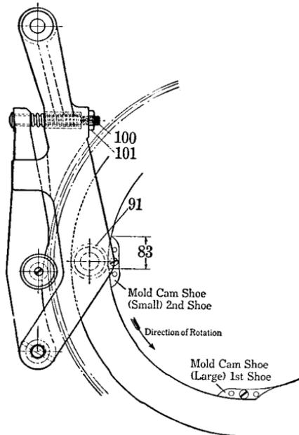
FIG. 19-32. View of the mold cam and driving gear when standing at right-hand side of machine, showing the resilient mold cam lever in position. For machines having this type of cam lever, adjustment for the proper clearance between face of mold and matrices when justification takes place is made by screw 100.
