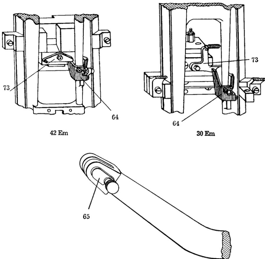
FIG. 14-32. View showing the toggle lock releasing mechanism and the first elevator lever link hinge pin. The releasing latch 64, which is attached to the first elevator slide contacts the locking toggle release lever 73 to release the toggle lock, thus allowing vise jaws to return to normal position.
