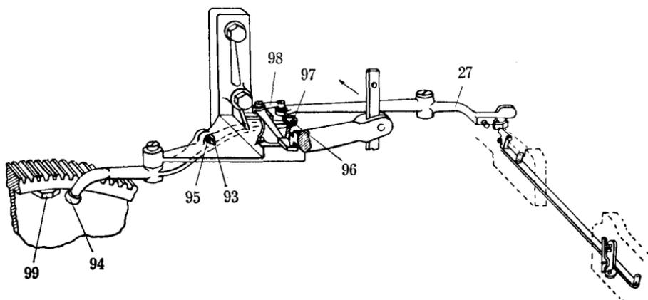
FIG. 20-32. View of the vise jaw safety mechanism.
