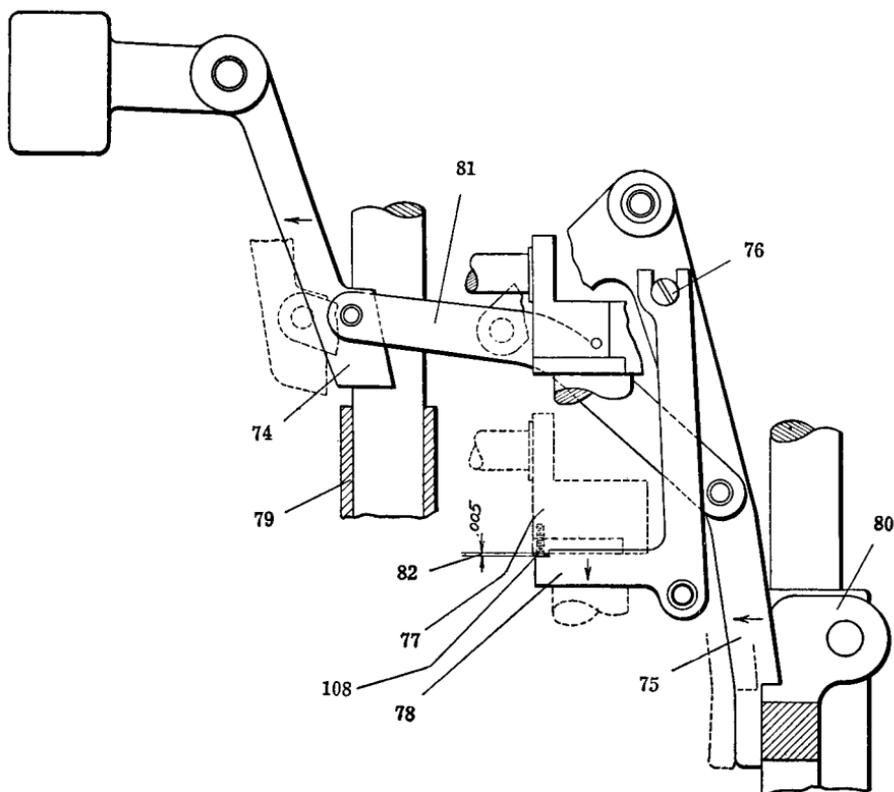
FIG. 17-32. Mechanism for controlling justification. This view shows the .005" clearance between the control rod 77 and the lever 78. It also shows the position the levers assume when the machine is being operated on quadding or centering and when the spaceband driver is prevented from rising.
